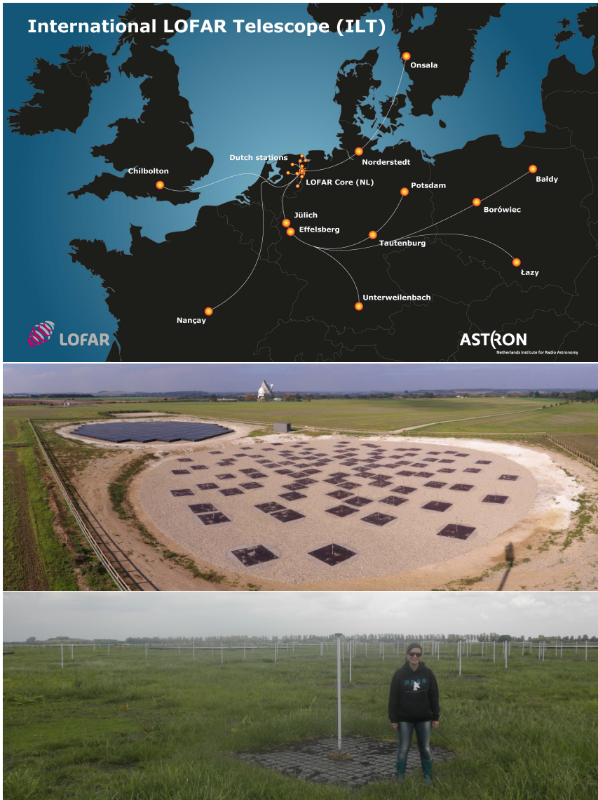
Figure 4: Top : The locations of LOFAR stations. The data in this thesis were taken before the stations in Poland were constructed, when the longest baseline was between Onsala and Nançay (1292km). Middle : The LOFAR-UK station at Chilbolton. The LBA antennas are in the foreground with the HBA antennas clustered together under a weather-protective covering behind the LBA. Bottom : Dipoles from an LBA station within the central core of LOFAR, with the author in the picture for scale.
