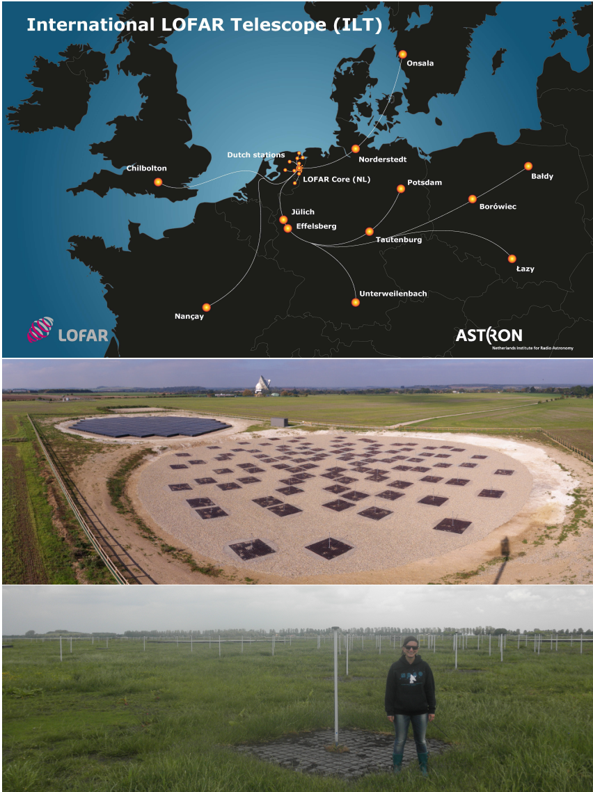
Figure 1.4: Top : The locations of LOFAR stations. The data in this thesis were taken before the stations in Poland were constructed, when the longest baseline was between Onsala and Nancay (1292 km). Middle : The LOFAR-UK station at Chilbolton. The LBA antennas are in the foreground with the HBA antennas clustered together under a weather-protective covering behind the LBA. Bottom : Dipoles from an LBA station within the central core of LOFAR, with the author in the picture for scale.
